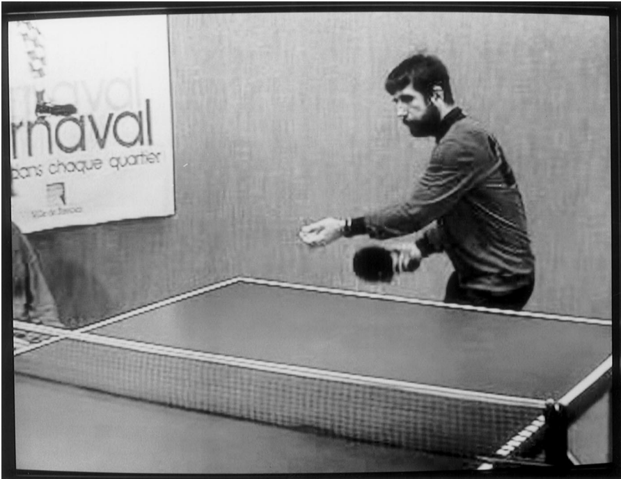
Fig. 5. Example of blurring. Table-tennis sequence coded at 1 Mbps. Most evident around the net and the surface of the table.
