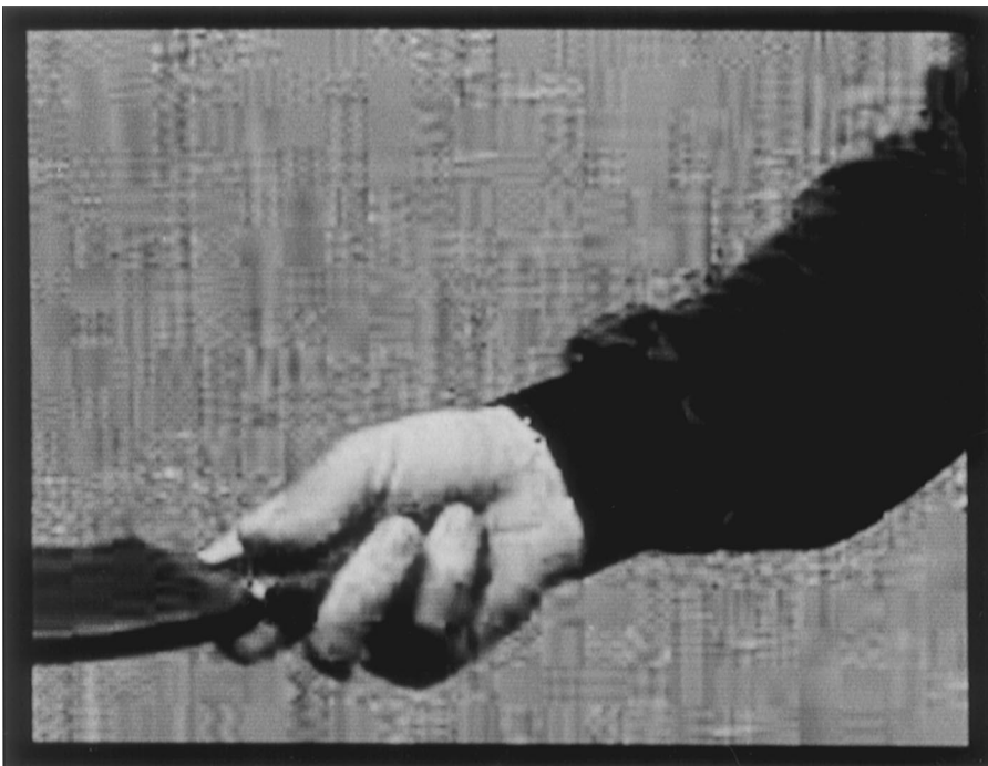
Fig. 20. Example of the high-frequency noise induced by MC mismatch around the boundaries of moving objects.
