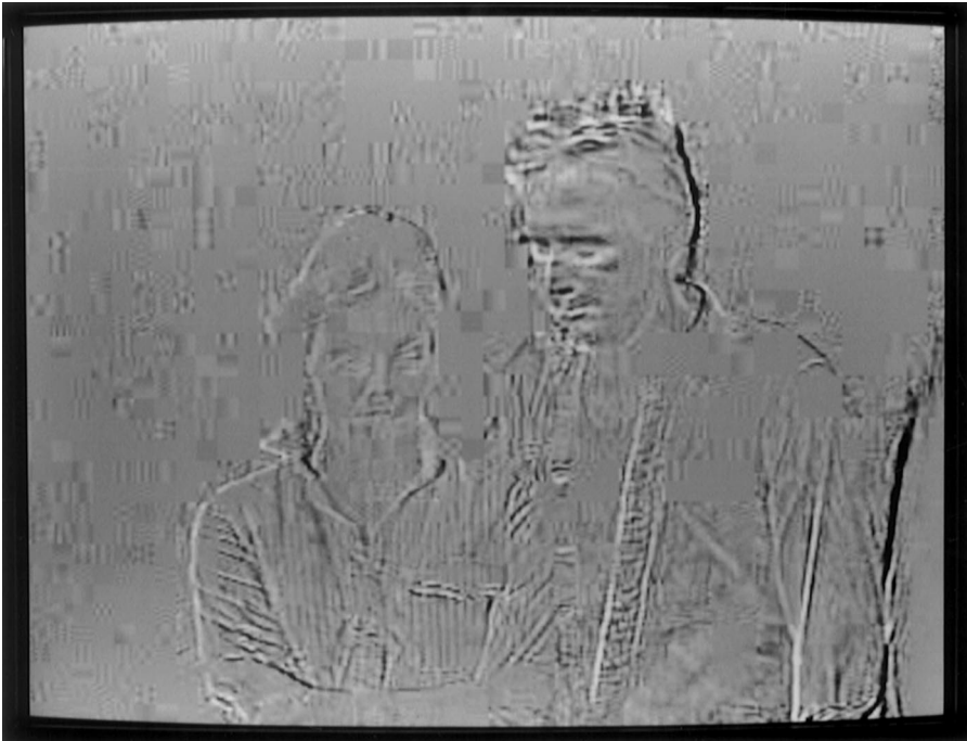
Fig. 25. Difference between frames 40 and 41 of the Sons and Daughters sequence. For the purpose of display, the difference is offset by + 128 and clipped to be within 0 and 255.
