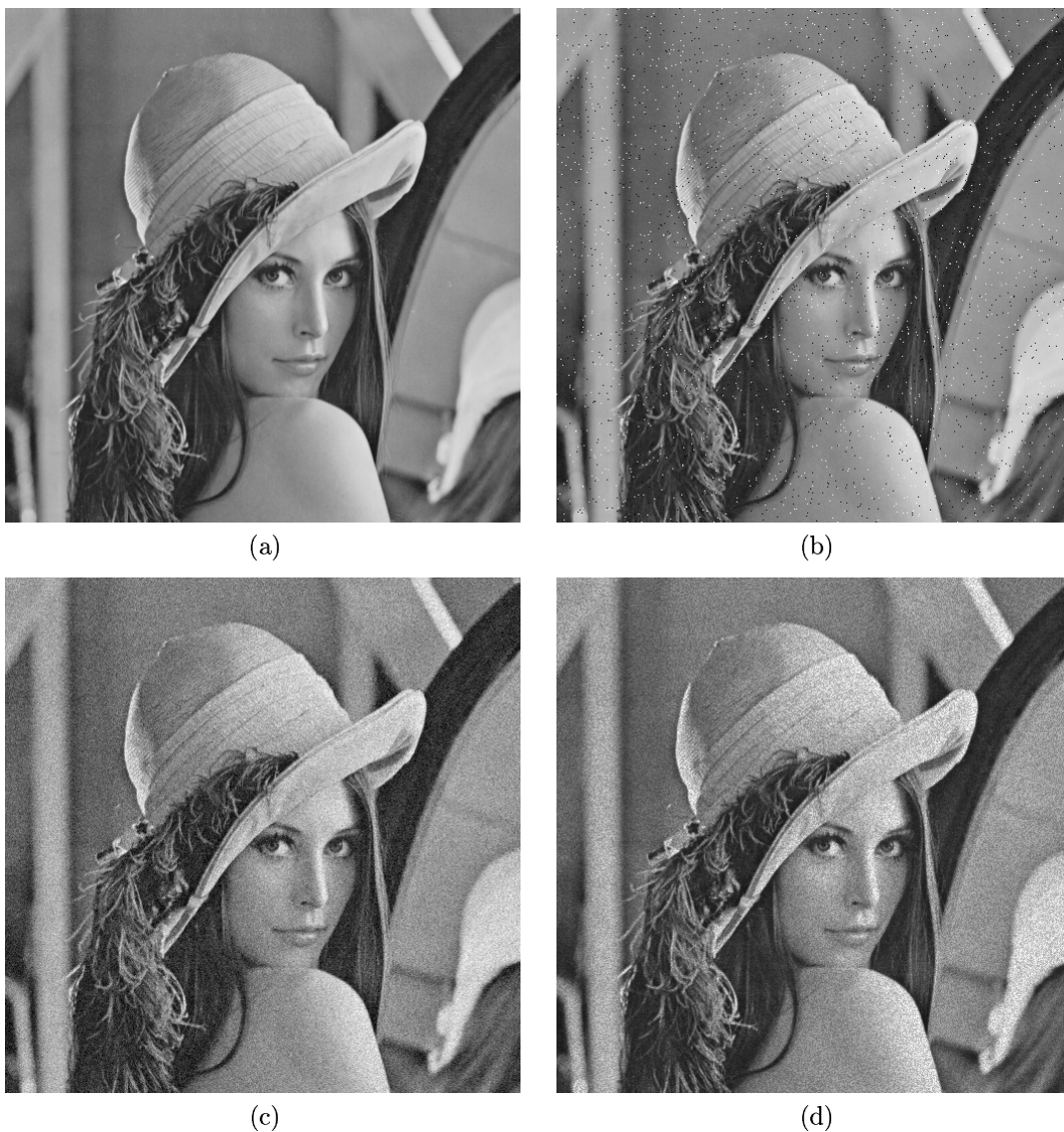
Fig. 1. Evaluation of "Lena" images contaminated by impulsive salt-pepper, additive Gaussian, and multiplicative speckle noises. (a) Original "Lena" image, 512 \times 512 , 8bits/pixel; (b) Salt-pepper noise contaminated image, MSE = 225 , Q = 0.6494 ; (c) Gaussian noise contaminated image, MSE = 225 , Q = 0.3891 ; (d) Speckle noise contaminated image, MSE = 225 , Q = 0.4408 .
