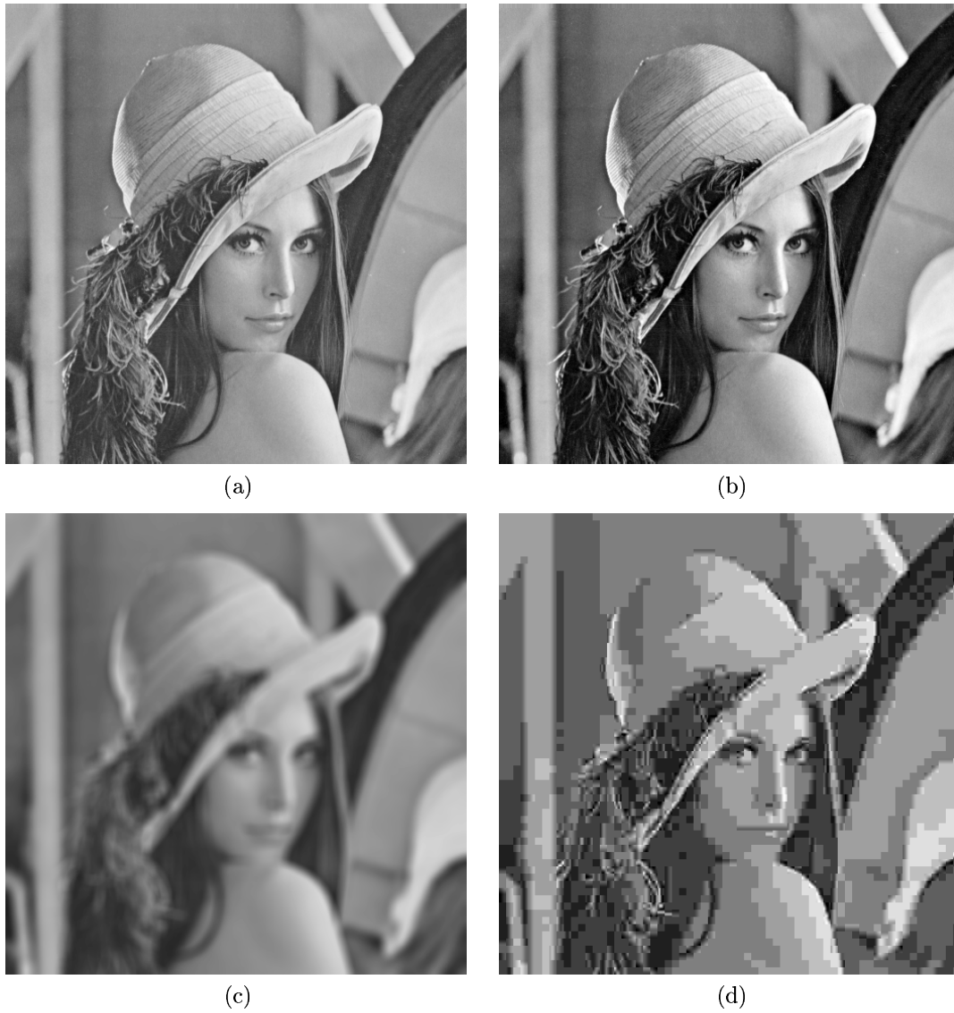
Fig. 2. Evaluation of "Lena" images distorted by mean shift, contrast stretching, blurring, and JPEG compression. (a) Mean shifted image, MSE = 225, Q = 0.9894; (b) Contrast stretched image, MSE = 225, Q = 0.9372; (c) Blurred image, MSE = 225, Q = 0.3461; (d) JPEG compressed image, MSE = 215, Q = 0.2876.
