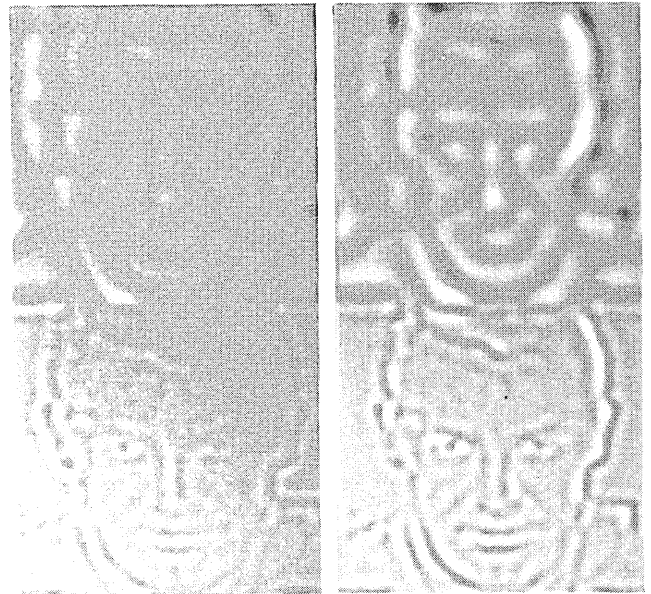
Fig. 2. Comparison between bandpass amplitude image (left) and local band-limited contrast image (right) for two spatial frequencies, 16 (top) and 32 (bottom) cycles per picture. Note the relative increase of contrast around the eyes and over dark areas in the original image (at left in Fig. 3 below).
