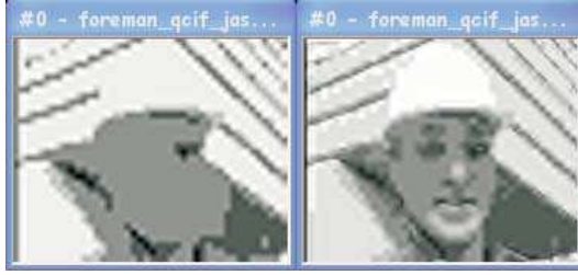
FIG. 7: First frame of Foreman QCIF encoded at 70 Kbps (left) and 135 Kbps (right)
