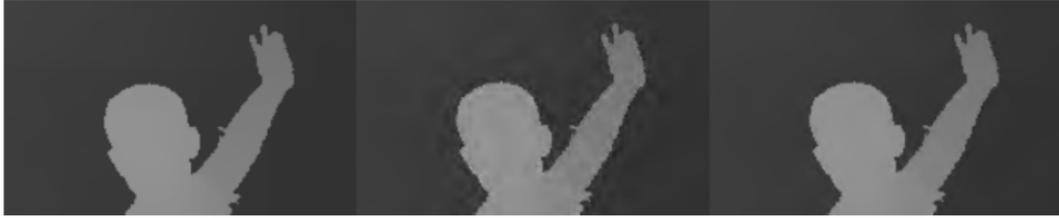
**Figure 2:** Ringing effect and result after the application of two dimensional joint bilateral filter to the 2D wavelet compressed depth map at 0.1 bpp
