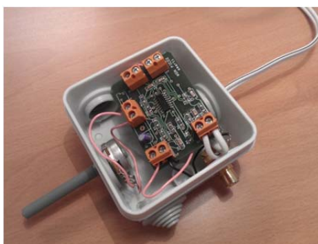
Figure 5. Signal conditioning and amplifying board prototype.
