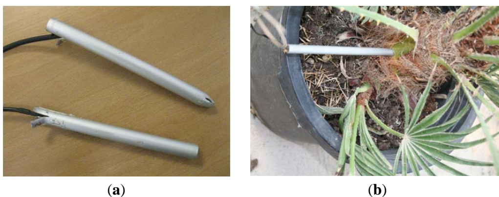
Figure 4. Open and Closed probes (a). Example of probe insertion (b).
