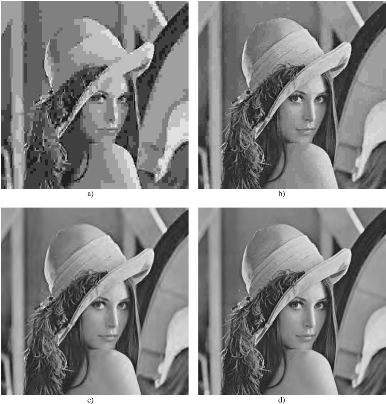
Fig. 1. Lena image compressed using JPEG a) and b), and using wavelets (LTW c) and d) (left column at very low bit rates (0.125 bpp approx.) and right column at low bit rates (0.25 bpp))
