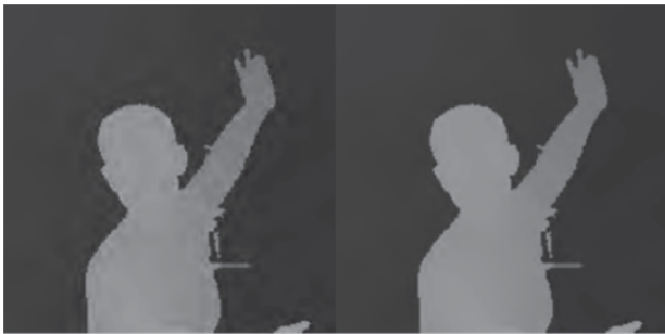
Fig. 2. . Ringing effect and result after the application of two dimensional joint bilateral filter to the compressed depth map in a frame of ballet sequence. Left image corresponds to part of the ballet sequence depth map compressed at 0.1 bpp. In the right image the de-ringing filter is applied on the compressed depth map.
