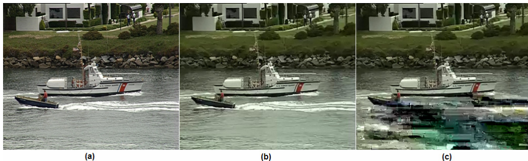
Figure 10. Subjective quality: (a) Coastguard original frame number 2191, (b) VP7 encoded-decoded, (c) VP7 reconstruction with packet losses.
