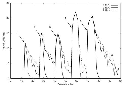
Fig. 9. Analysis of error propagation by simulating an increasing number of entirely lost frames
