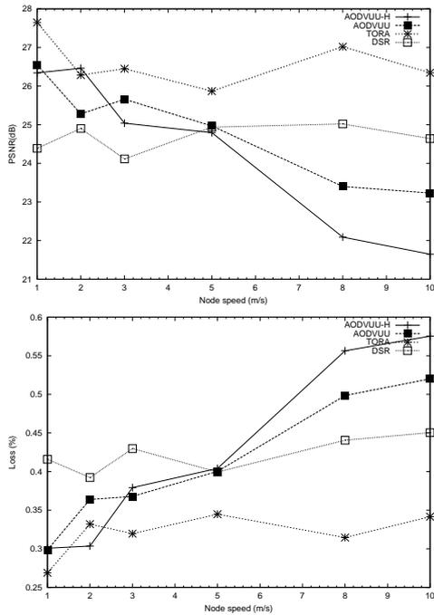
Fig. 3. Evaluation of different routing protocols for varying mobility in terms of packet losses and perceived PSNR for the video test sequence
