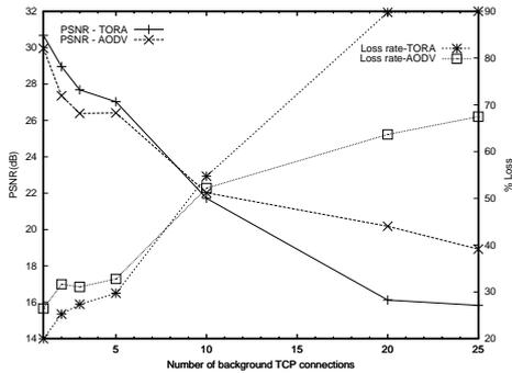
Fig. 4. PSNR and packet loss rate performance for a variable number of background TCP connections
