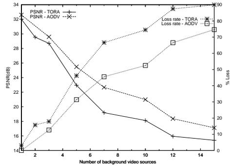
Fig. 5. PSNR and packet loss rate performance for a variable number of background video connections
