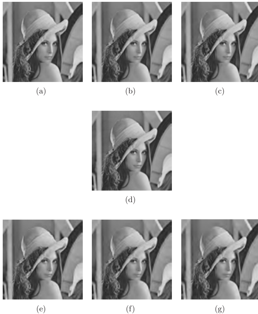
Figure 2.10: Lena compressed at 0.125 bpp and 0.0625 bpp - (a,e) LTW_RCi2%; (b,f) SPIHT; (c,g) JPEG 2000; and, (d) Original (not compressed)
