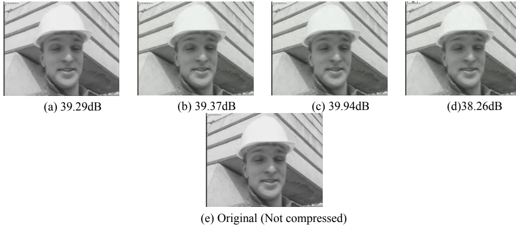
Figure 3. Foreman sequence (QCIF) compressed at 1012.16Kbps (Frame 14). a) H264 b) JPEG2000 c)M-LTW d) M-LTW_Int and e) Original (not compressed)
