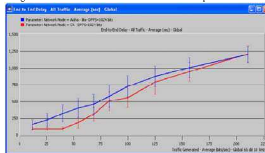
Fig. 4. Delay vs. Load: Results from original authors.
