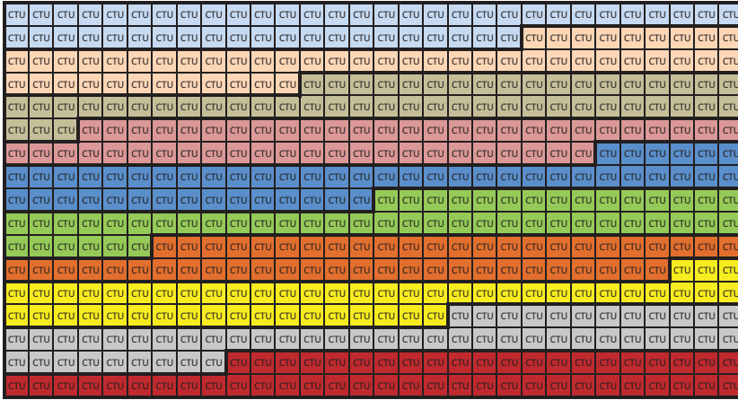
Fig. 1 Division of a full-HD frame (1920x1080 pixels) into 10 slices (of 51 CTUs each)
