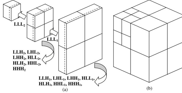
**Fig. 1.** Overview of the 3D-DWT computation in a two-level decomposition, (a) following a frame-by-frame scheme as shown in Fig. 2; or, (b) the regular 3D-DWT algorithm
