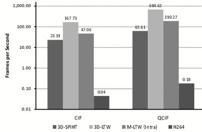
Fig. 7. Execution time comparison of the encoding process
