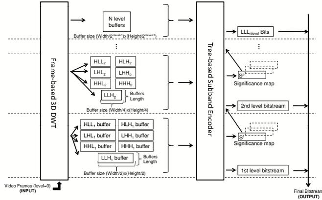
**Fig. 4.** Overview of the proposed tree-based encoder with efficient use of memory
