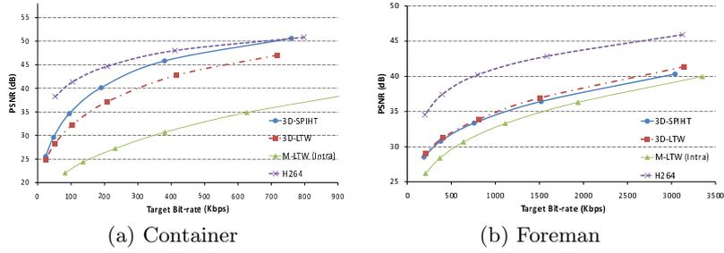
Fig. 6. PSNR (dB) for all evaluated encoders for a) Container sequence in QCIF format and b) Foreman sequence in CIF format
